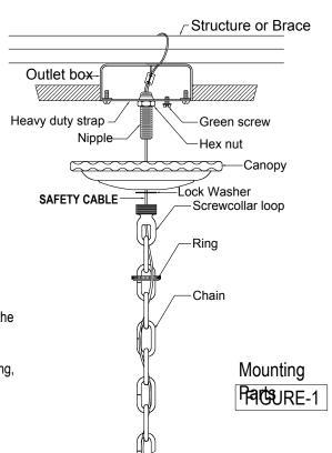
**4.** Open the end links of the chain and attach the chain to the screw collar loop. Hang the fixture on the chain at the desired height. Remove the excess chain close all links. Unscrew the threaded ring from the screw collar loop. Allow the ring and canopy to slide down the chain to the top of the fixture.
